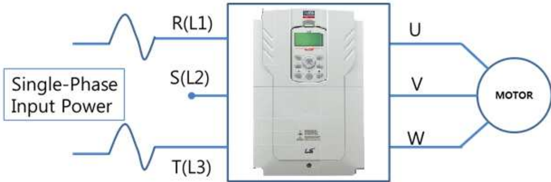
Figure-3 Terminal Wiring Diagram
